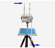
The hose delivered with BiVOC2V2 can be connected to the outlet of the sound suppressor to increase the distance between air inlet and outlet of the sampling air nearly indefinitely.
