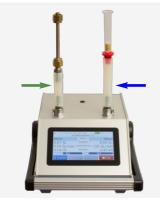
The photo shows the DNPH adapter (blue arrow) in operation on the right channel of BiVOC2V2.
