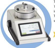
The high-performance air sampling head **LKS100** with a nominal flow rate of 100 l/min is available for air sampling of cultivable particles on culture media in 90-mm standard Petri dishes.
