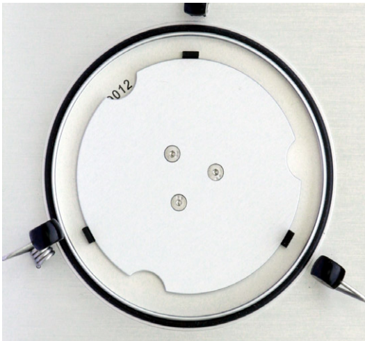
Figure 6 Centering mechanism narrow, disk in position 12
