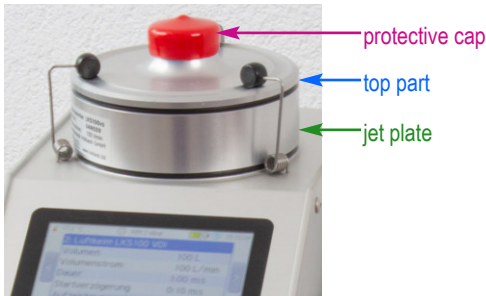
Figure 38 The air sampler's components
