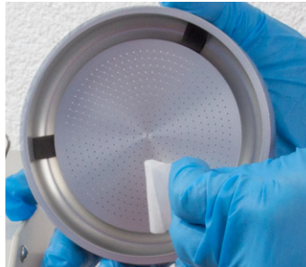
Figure 45 Clean the bottom of the jet plate
