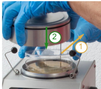
Figure 49 Remove lid of petri dish, place air sampler
