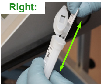
Figure 61 Position of the slide when taking or inserting it
