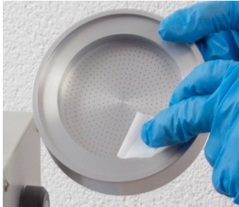
Figure 44 Clean the top of the jet plate
