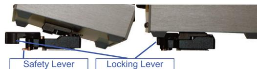
Insert device diagonally and push downwards
