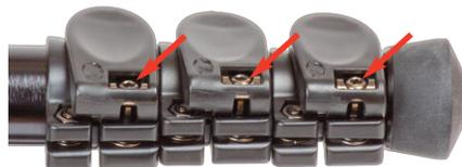
If the lever is very hard to operate, the screws are too tight.
