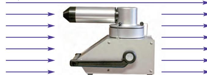
Sampling in external air flow with transverse adapter and inlet nozzle
