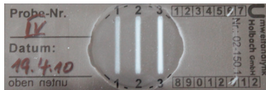
Fig. 38 Totally overloaded particle tracks (not suitable for analysis)
